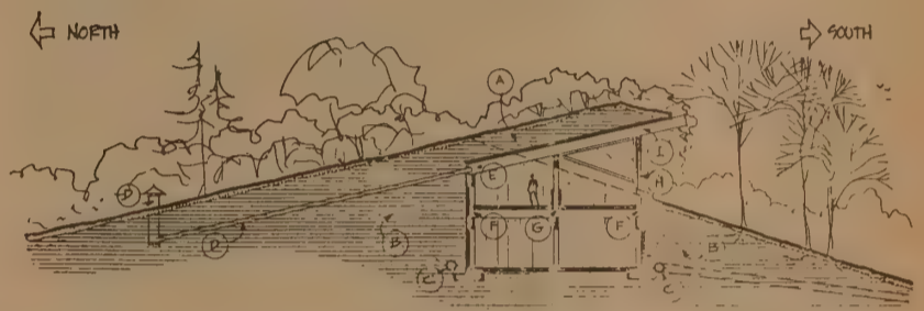
7-17-72 DRAWN BY MALCOLM B. WELLS OF MALCOLM B. WELLS PROFESSIONAL ASSOCIATION AN EARTH-COOLED, SOLAR-HEATED HOUSE. 1/16" = 1'-0" SECTION
